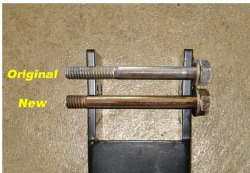
New 8mm, Class 10.9 bolts are available at Advanced Automotive Technologies Corporation 262-673-4077 <http://superformance.org/mountupgrade> or you can use 5/16" Grade 8 bolts from suppliers such as [www.aircraftspruce.com](http://www.aircraftspruce.com) part number AN5-27A
